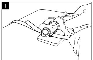
Squessze the handle to lift support frame. While in this position, move the tool and slide the strap under the feedwheel. The strapping material is now locked and ready to be tightend.
