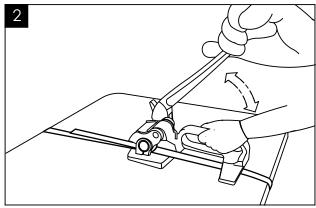
Hold the tool with your left hand and pump the handle until the straps are suffciently tight.Don't over-tighten the straps as damage may occur to the tool and object being strapped.
