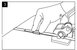
Place the seal open side down over both straps in front of the tool.
