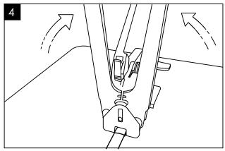
Open the sealer fully open position, put the sealer on the top of the seal, press the sealer handle together to fully crimp the seal, then remove the sealer.
