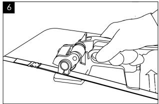
Compress down the handle to lift the feedwheel. Slide the tool away from the strapping materal. Cut excess strap with a steel strapping cutter.
