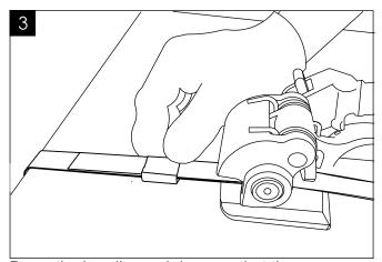
Press the handle pawl down so that the handle can be released.
