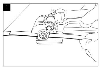
Squessze the handle to lift support frame. While in this position, move the tool and slide the strap under the feedwheel. The strapping material is now locked and ready to be tightend.
