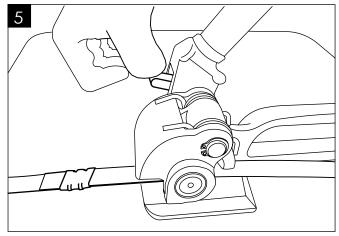
Place the seal open side down over both straps in front of the tool.
