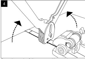
Open the sealer fully open position, put the sealer on the top of the seal, press the sealer handle together to fully crimp the seal, then remove the sealer.
