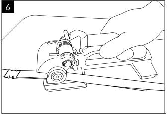
Compress down the handle to lift the feedwheel. Slide the tool away from the strapping material. Cut excess strap with a steel strapping cutter.
