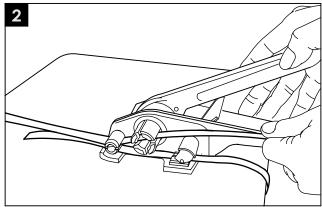
Release the handle and base to secure strap. Feed the other end of strap through the slot of cutter and windlass. Pull strapping as tight as possible by hand.
