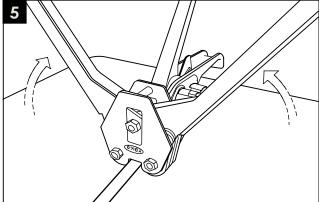
Open fully the sealer and place it on the top of seal. Close the sealer to crimp tightly the seal and stap.
