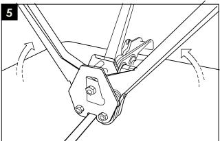
Open fully the sealer and place it on the top of seal. Close the sealer to crimp tightly the seal and strap.
