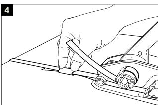
Place seal open side down over both straps in front of the tool.
