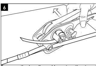
Squeeze the handle and base together to cut the strap and then slide the tool to the right.
