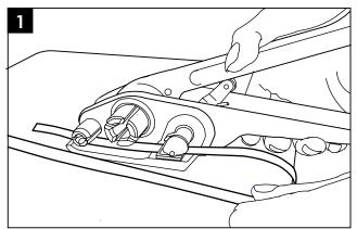
Wrap the strap around the container as shown. Squeeze handle and body together to lift the leg so the strap can be placed under the gripper plate and cutter.
