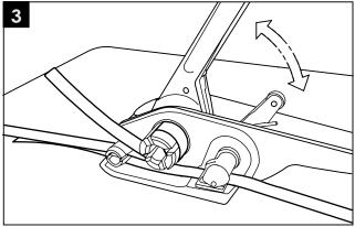
Hold the tool with left hand. Move handle back and forth until strapping has reached desired tension.
