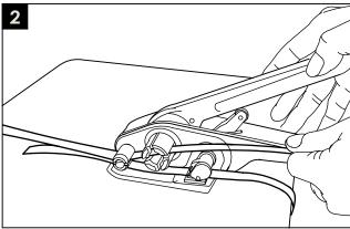
Release the handle and base to secure strap. Feed the other end of strap through the slot of cutter and windlass.Pull strapping as tight as possible by hand.
