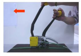
6. Hold the tensioning handle and push the sealer handle forward to close the seal.
