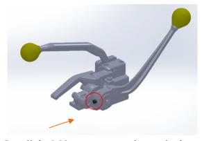
1. Install the M6 cap screw on the tensioning handle before use.
