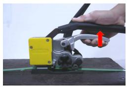
7. Pull the cutter handle up to cut the strap. Slide the tool out to the right, and then release the handle.
