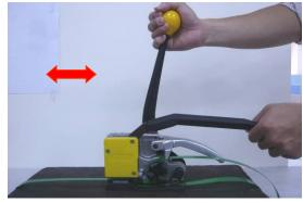
5. Move the tensioning handle back and forth to tighten the strap.
