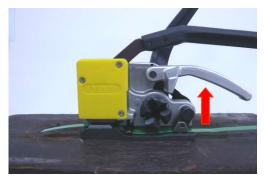
3. Put strap around the packed object and pull the cutter handle up to place the strap under the foot. Pass the strap through the seal and release the handle.
