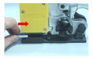
2. Slide a seal inside the slot of tool.
